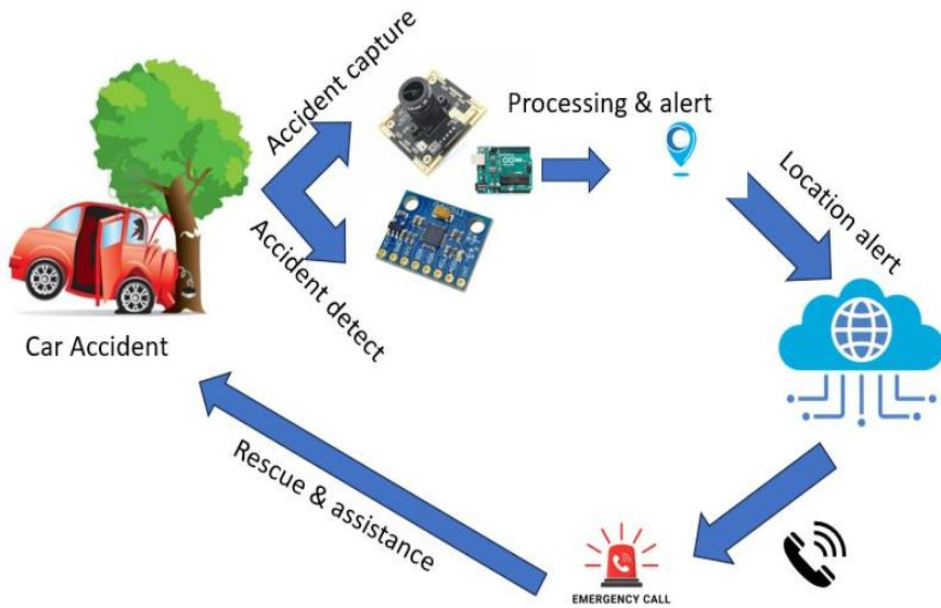
Vehicle motion is tracked continuously by onboard sensors onboard a vehicle. Upon an accident, the system detects the impact, captures visual evidence of it, processes the data, and sends real-time alerts with the location of the accident to emergency services through cloud connectivity.
