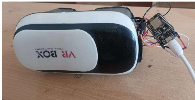
Figure 4: Hardware prototype showing Mask, ESP8266 NodeMCU Board
