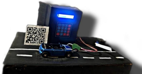
Fig 3: PETROL CONNECT: An IoT enabled smart card and QR code based secure fuel ATM
