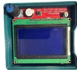
Fig 4.2 Custom LCD Holder for User Interface Control
