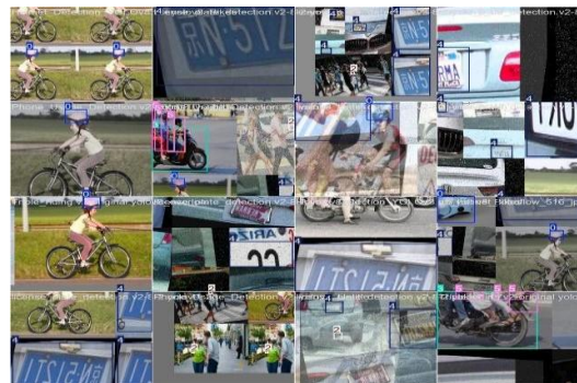
Fig. 5. YOLOv8-based detection of multiple traffic violations
