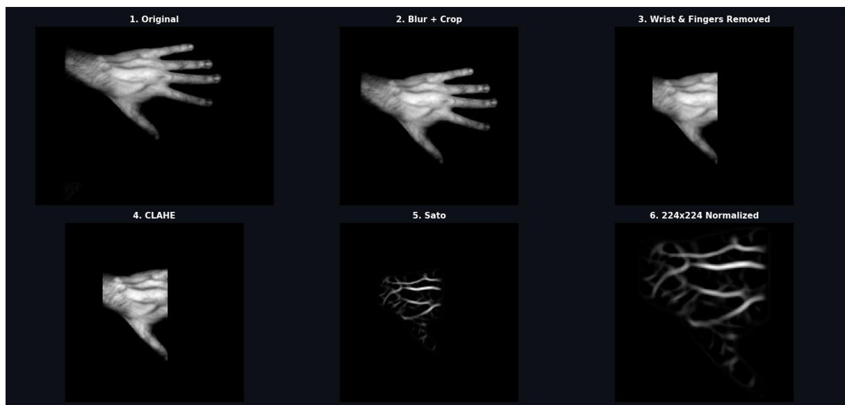
Fig. 1 Preprocessing pipeline for dorsal hand vein enhancement illustrating six representative stages from the complete ten-stage pipeline: (1) Original NIR image, (2) Gaussian blur and smart crop, (3) Wrist and finger removal, (4) CLAHE contrast enhancement, (5) Sato vesselness filtering, and (6) Final 224×224 normalized output.
