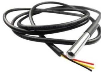
Fig. 6. DS18B20 Waterproof Digital Temperature Sensor.
