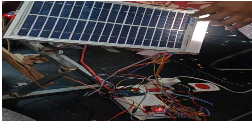
Fig. 4. Assembled Prototype with Tracking Frame and Controller Output.
