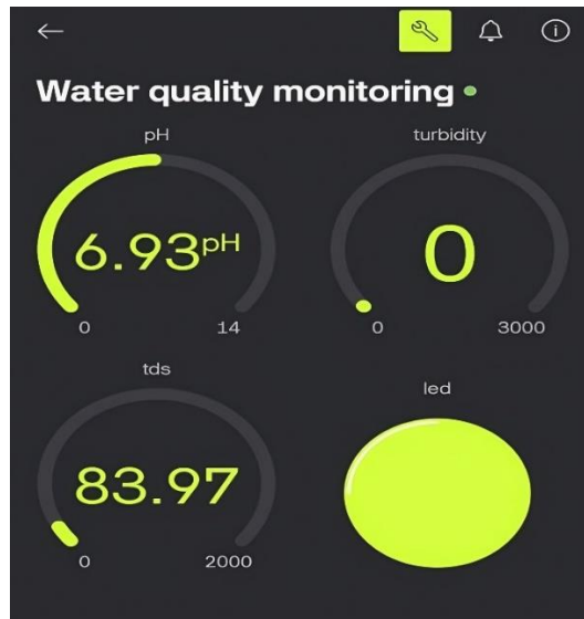
Fig.4: Blynk Dashboard Showing Parameters Of Water Quality
