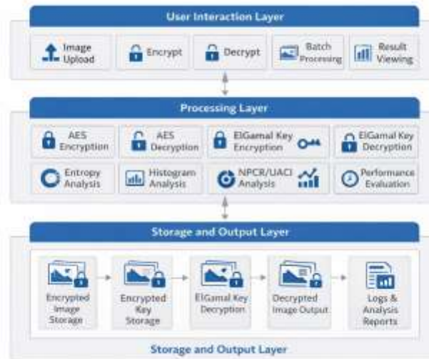
Fig. 1. Proposed Hybrid ElGamal-AES System Architecture
