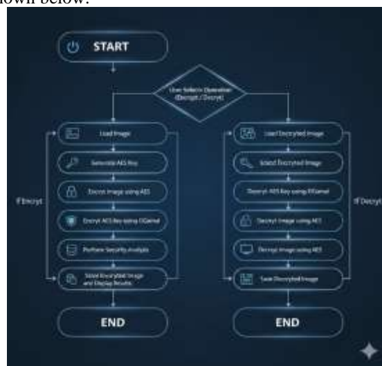
Fig. 2. Hybrid Encryption and Decryption Workflow
