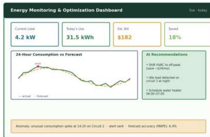
Fig. 4. Implementation view of the dashboard showing consumption indicators, forecast overlay, anomaly alert, and AI savings recommendations.
