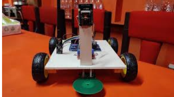
Fig.1 model of autonomous/tele-operated landmine detection robot
