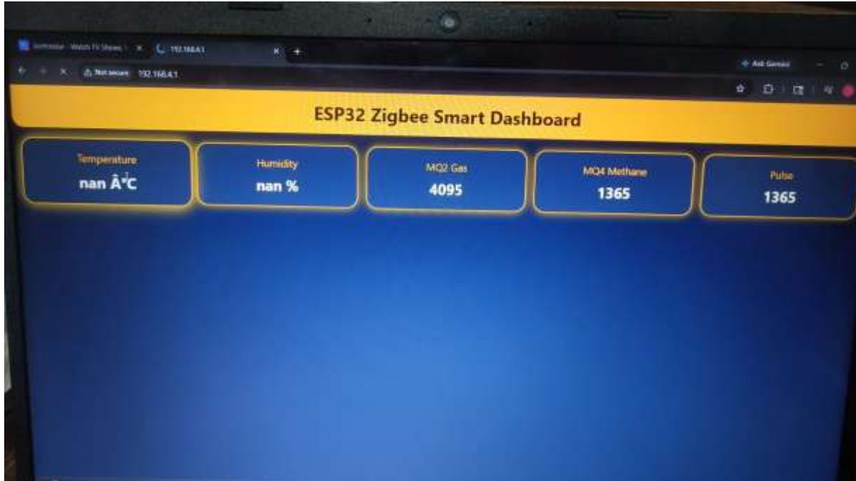
Fig. 1. Design and Implementation of ZigBee-Based Smart Helmet with Real-Time Monitoring Dashboard for Miner Safety
