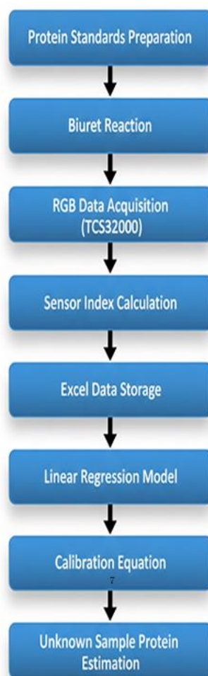
Fig. 2. Flowchart of the Proposed Protein Detection System
