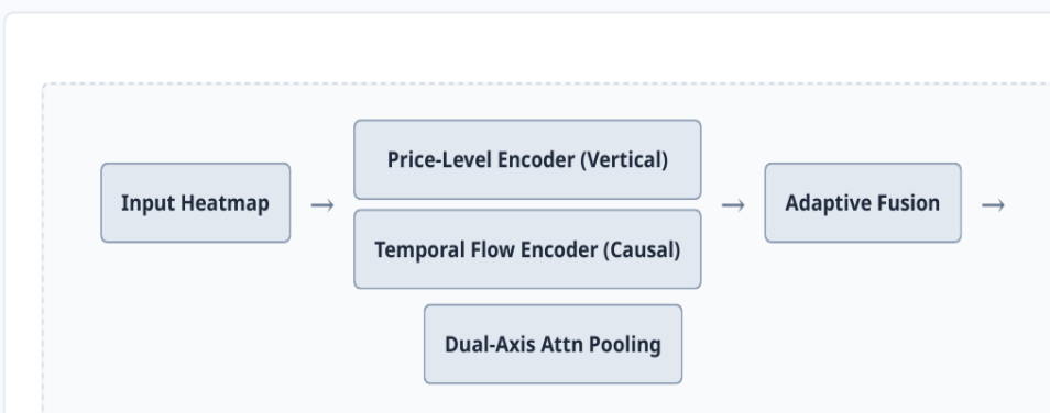
Figure 4. Proposed DAFNet architecture with separate price-level and temporal-flow encoders, adaptive
